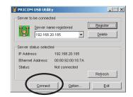
Your PC and USB scanner has been connected over the network with the PRICOM. Activate the scanner's TWAIN utility to use it as a network scanner.
