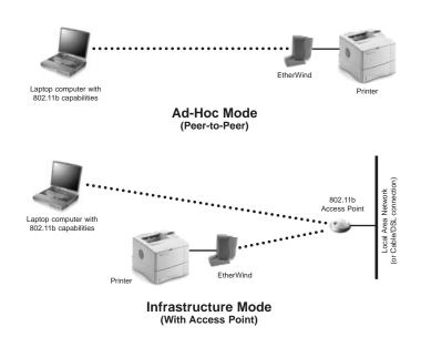
The print server operates at speeds of up to 11 Mbps on any IEEE 802.11b wireless compatible network. Your printer can be simultaneously connected to your PC or Macintosh via the USB port.
